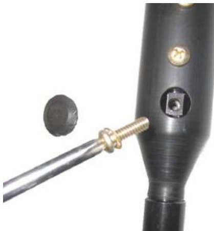
Fig. 6 – Disconnecting activation cable
