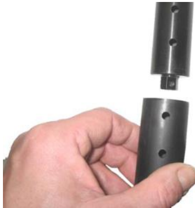
Fig. 8 – Rocket Removal from Pedestal
