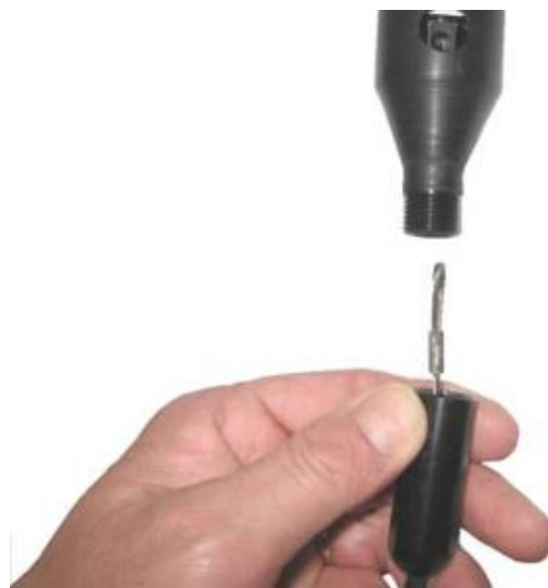
Fig. 7 – Cone adapter removal
