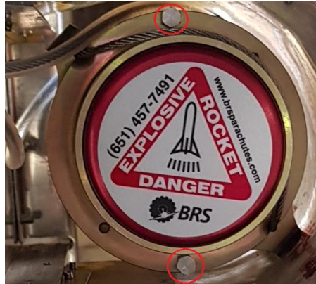
Fig. 10 – Disconnecting the pick-up collar
