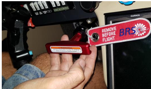
Fig. 2 – Activation Handle, secured
