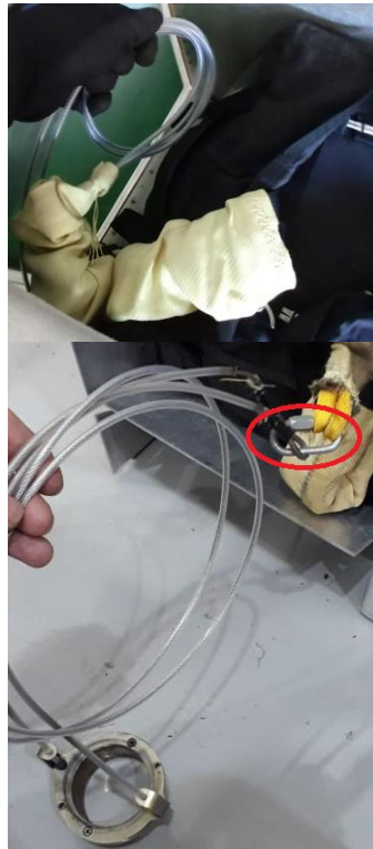
Fig. 5 – Removal of canister backplate
